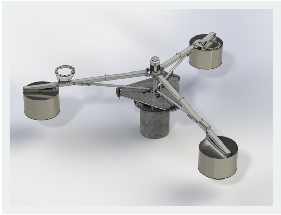
NSA2-15 retrofit for Envirex 15 HP Floating Aerator CHESTER, VA
